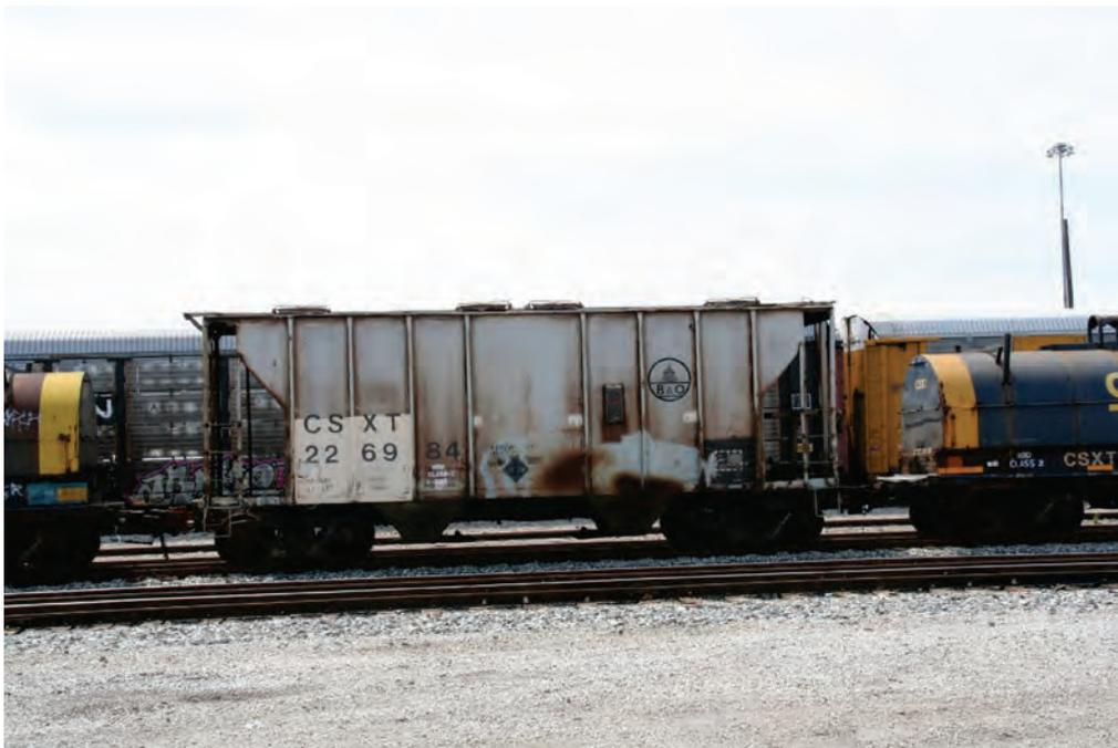
**CSXT 226984 is a two bay, four loading hatch hopper car built by Pullman Standard in 1965 for the Baltimore & Ohio Railroad. She is seen at Evansville, Indiana, in 2011. Her dimensions are 40 feet 6 inches by 10 feet 7 inches by 14 feet 10 inches. With an internal capacity of 2,700 square feet, she can carry 205,000 pounds of goods.**
