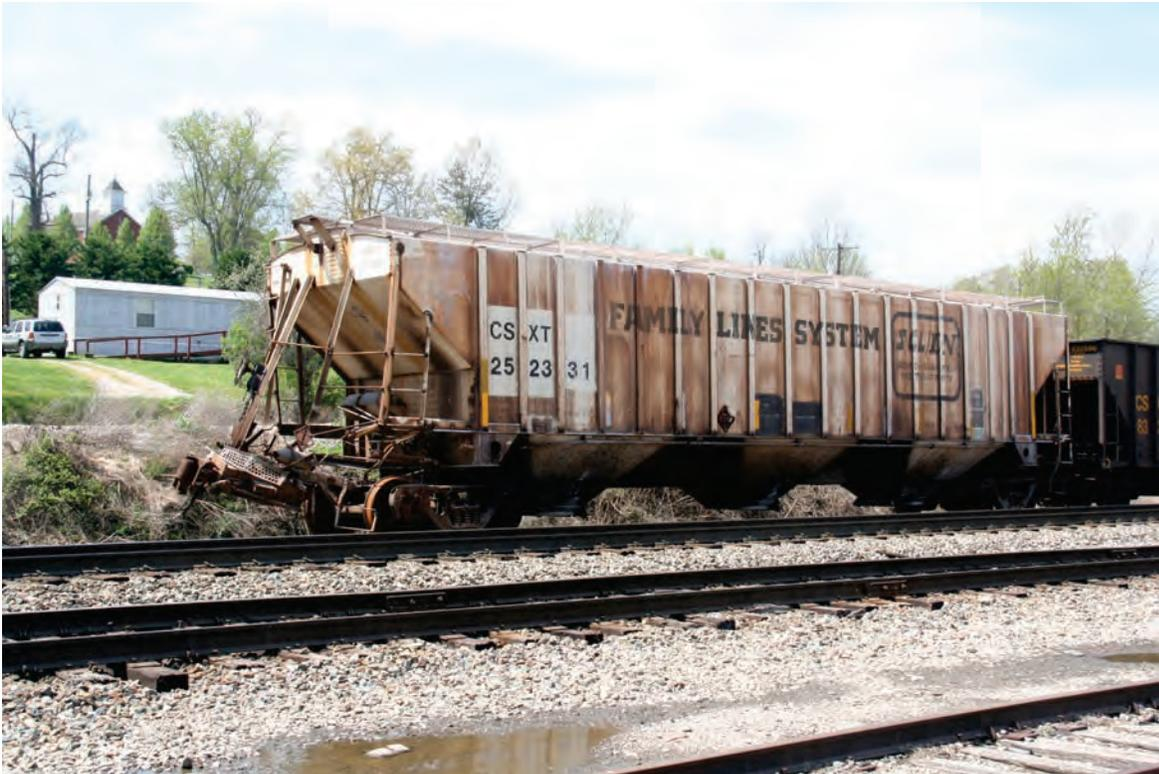
**Above and below is CSXT 252331, a three bay, ex Family Line, 1979 Pullman Standard built covered hopper. She sits on the siding at East Bernstadt, Kentucky, in June 2013, having suffered coupler failure on her “A” end while traveling over Crooked Hill.**
