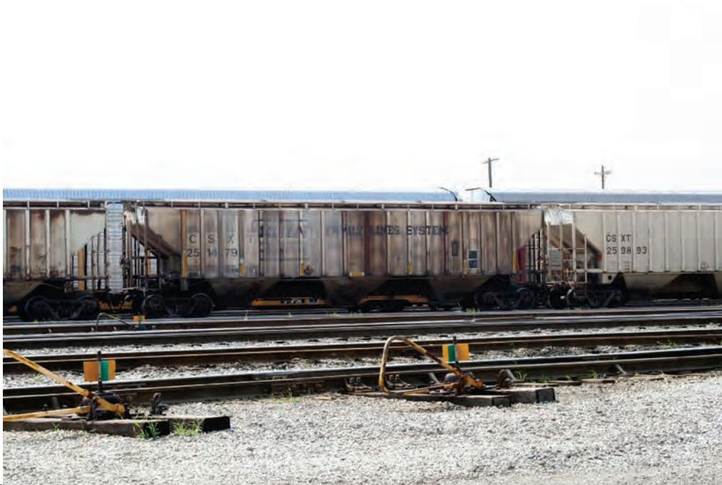
**CSXT 251479, still in Family Line paint, is the former SCL 242020. Seen here at Columbus, Ohio, in 2011, she is 59 feet 11 inches long, 10 feet 7 inches wide, and 15 feet tall. With a cubic capacity of 4,759 cubic feet, she can carry 201,000 pounds of goods.**
