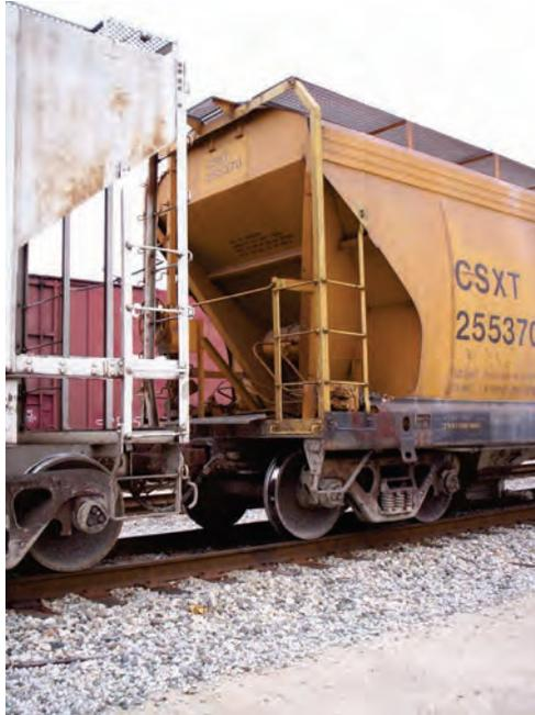
**On this page and the next are four close-up photos of the three bay, gravity unloading, covered hopper CSXT 255370, which is featured on the cover of this issue. This former Chessie System car was built in 1981 for the C&O by American Car & Foundry Company. She is 54 feet 7 inches long, 10 feet 8 inches wide, and 15 feet 6 inches tall. She can carry 198,000 pounds of goods. The photos were taken in 2011 at Barr Yard, Chicago.**
