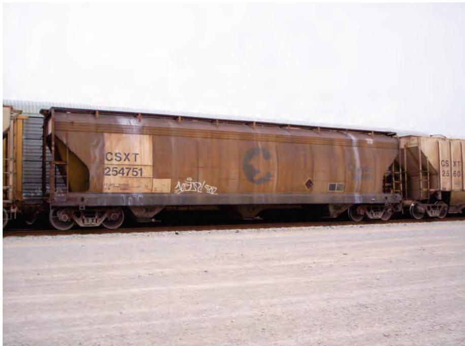
**CSXT 254751, built by AFC, is a sister car to CSXT 255181. Note the difference in weathering between the two cars and the manner in which the Chessie reporting marks were obliterated by CSXT.**
