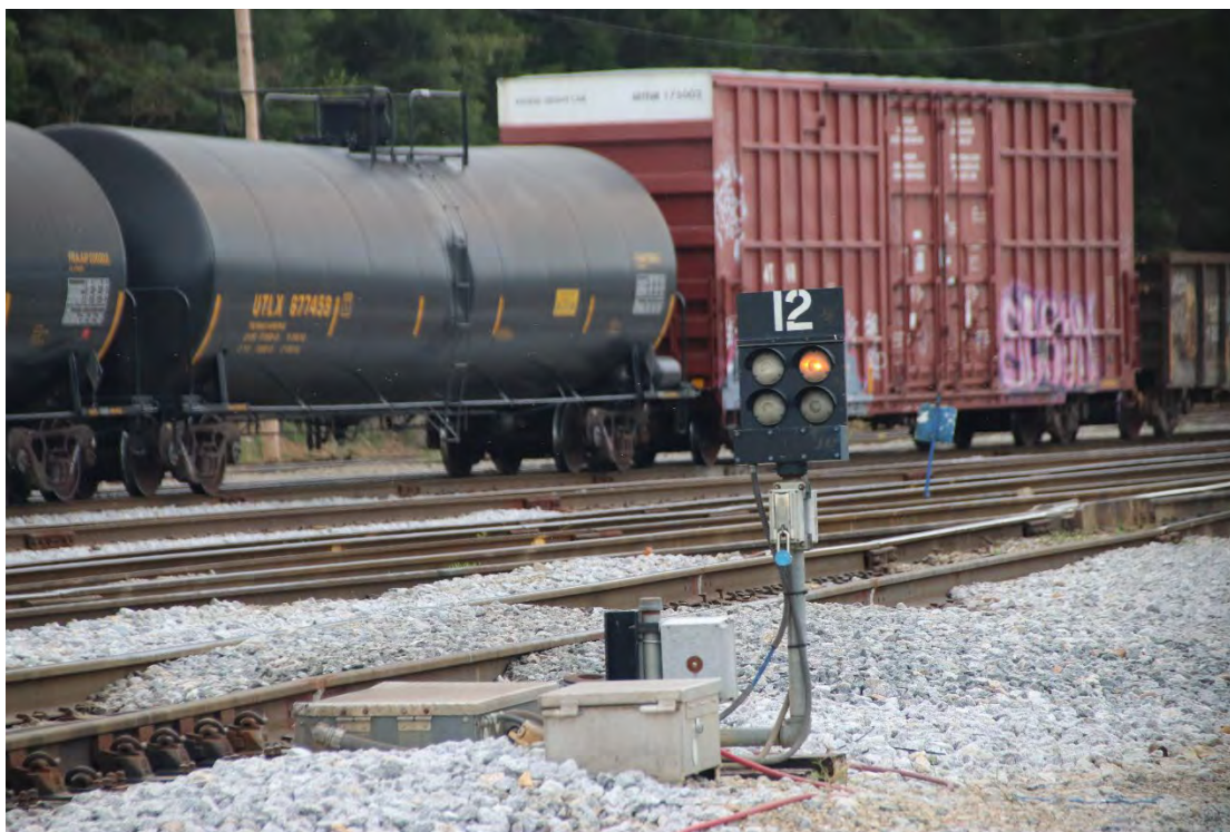
Above and below: Close-up of Wauchatchie Yard air powered switches.
