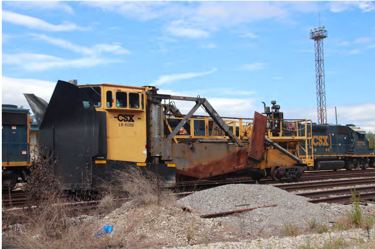
Above and below: Views of L&N 41288, a Jorden Spreader
