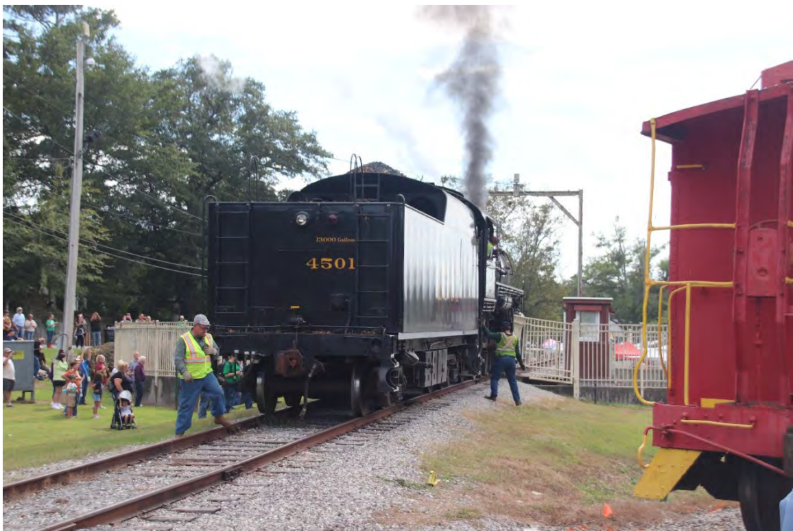
Turning Southern 4501 on the turntable at Summerville.
