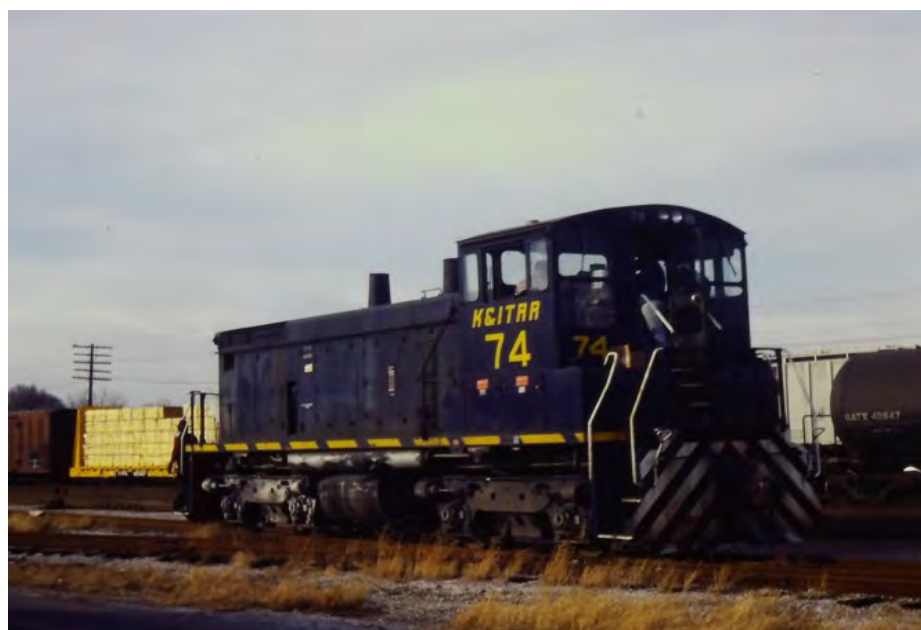
K&IT 74 a EMD SW 1500 purchased in 1971 is seen at Illinois Central Oak Street Yard. Note the trainman on the front footboard and the trainmen standing on the steps leading into the cab.
