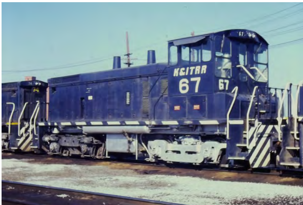
K&IT 67 was the first EMD SW1500 switcher purchased by Kentucky & Indiana Terminal Railroad. Bought in 1966 she later became Southern 67, Norfolk Southern 67, Parker Service 67, ILSX 67, Progress Rail 67. Note K&ITRR lettering has been moved from the hood to the cab.
