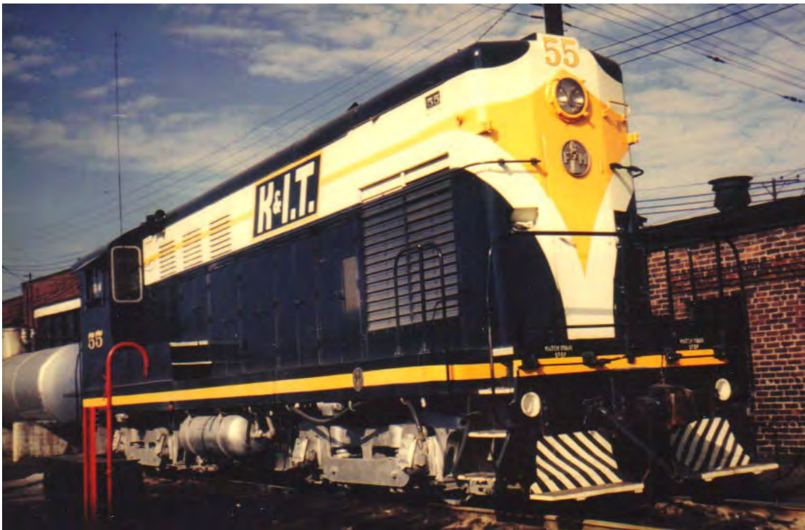
K&IT 55 was a Fairbank Morris FM 10-44 purchased in 1949 and sold in 1973 to Precision National. Note the FM medallion below the headlight and the running boards.
