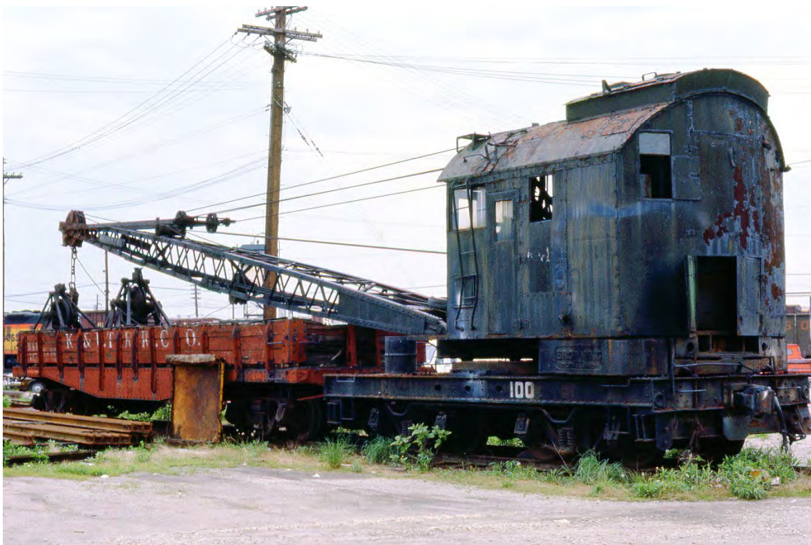
Above and below: steam powered crane K&IT100 and its boom car.
