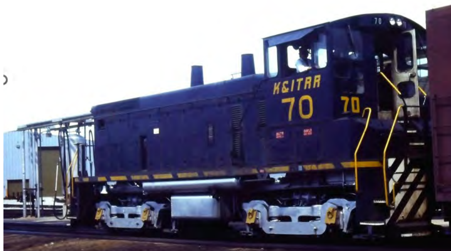
K&ITRR 70 was a EMD SW1500 purchased in 1968. She is seen here pushing a boxcar into a siding of one of Louisville's trackside industries. Engineer is looking back alongside his consists to see singals of his traiman. K&ITRR 70 later became Southern 70, Norfolk Southern 70, and Wisconsin Central 1560
