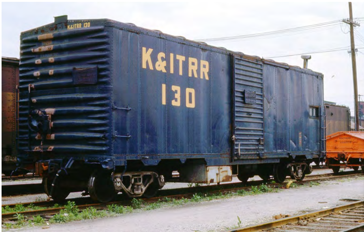
K&ITRR 130 was a boxcar converted to Maintenance of Way use. Note the window in the side of the boxcar and the smoke stack jutting out of the roof. K&ITRR has removed the boxcar's roof walk. Note the location of the former ladder. Also the hand brake has been moved down from the roof line to ground level. An orange Southern Railway scale car sits just beyond K&ITRR 130.
