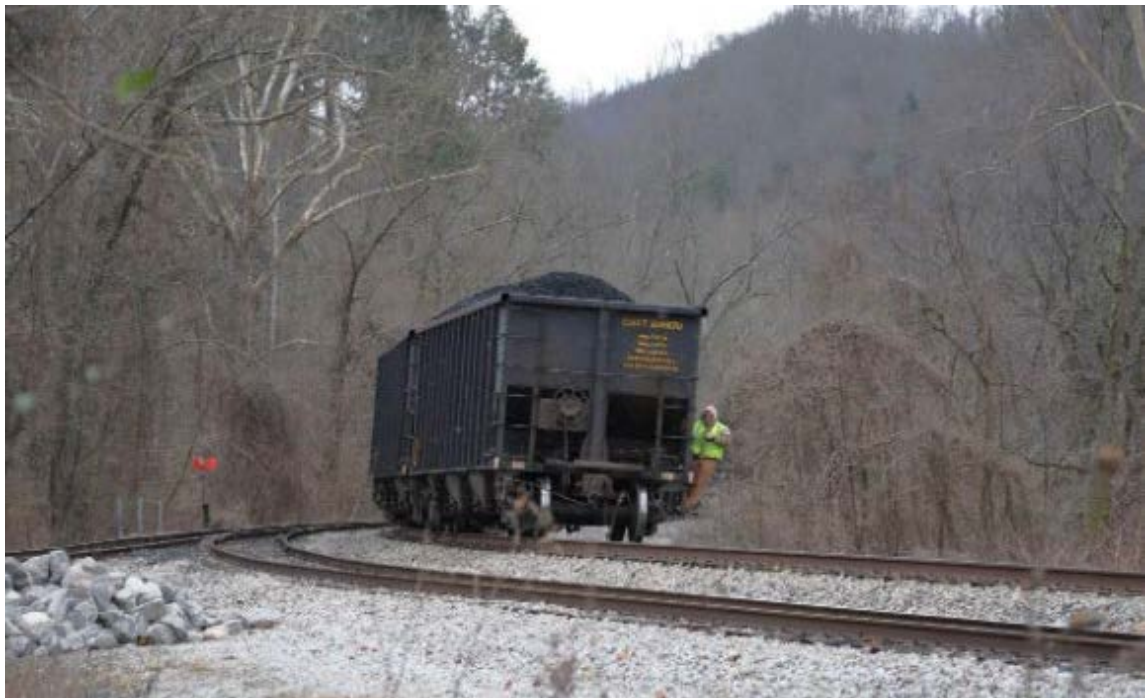
R615-29 then shoves the first cut down the main line.
