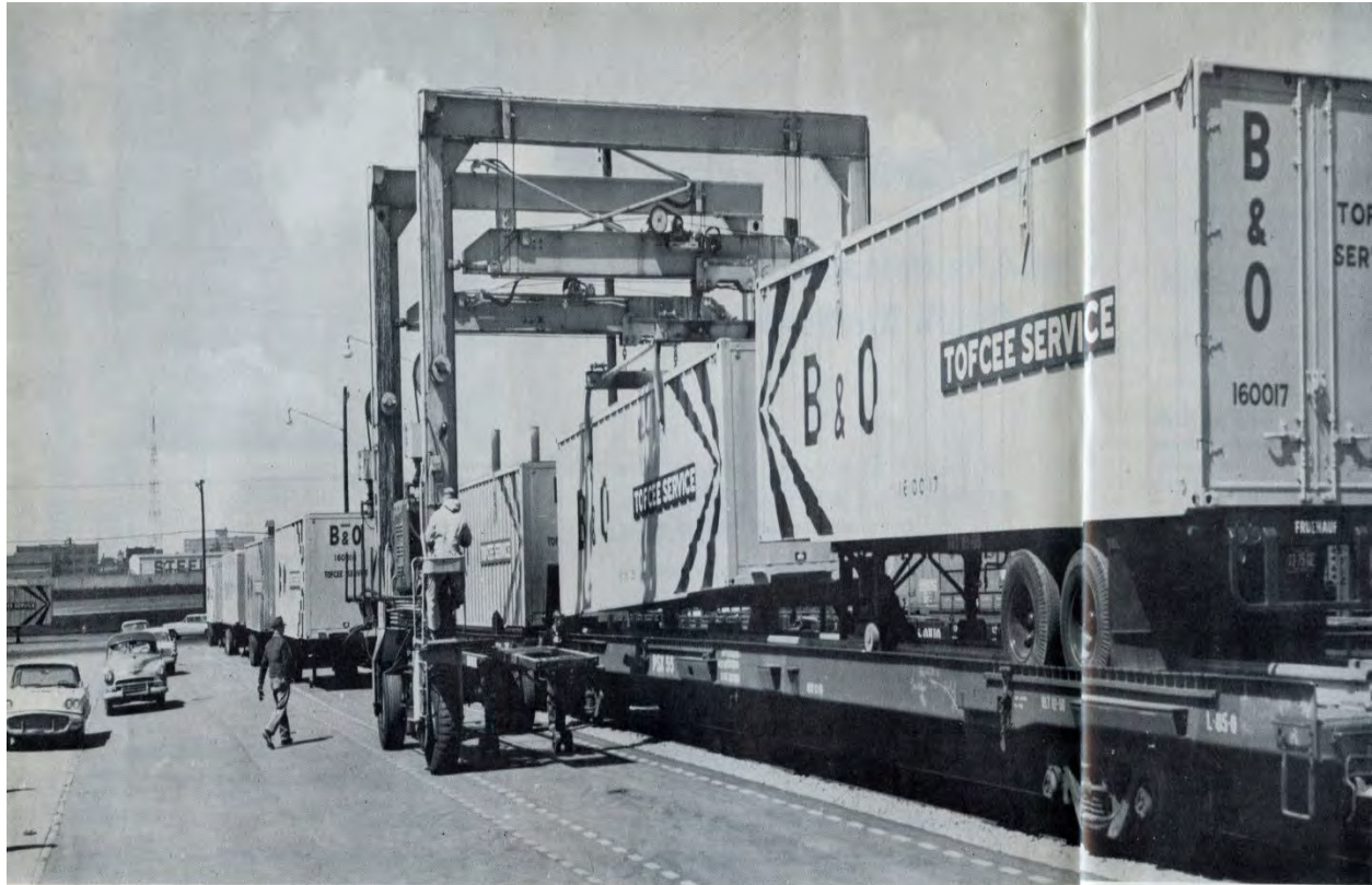
Travelift crane operator deposits demountable body onto flat car at B&O's East St. Louis TOFCEE handling facility. At present B&O has 255 demountable bodies in piggyback service, and 405 wheeled vans. An additional 100 vans are now on order
